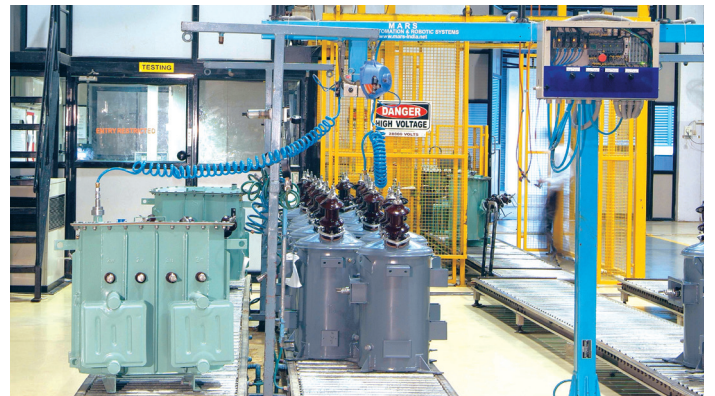
Oil leakage testing
